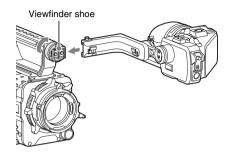
2 Tighten the fixing ring after determining the left and right position of the viewfinder, then connect the viewfinder cable to the VF connector of the camcorder.
