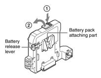
Insert the projection of the battery adaptor into the slot on the rear of the camcorder (1), then lower the ejection lever (2).
